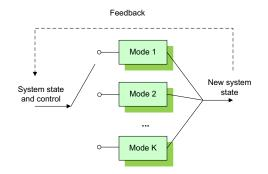
Fig. 2: An illustration of hybrid systems.
